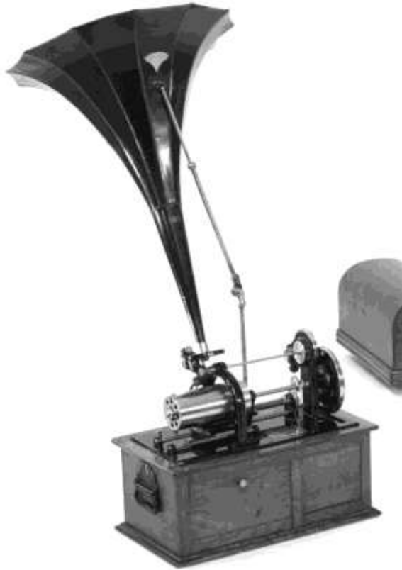
Left: An Edison Kinetograph (1912-13). The large wheel on the right side of the mechanism is where the synchronizing cord was attached.
