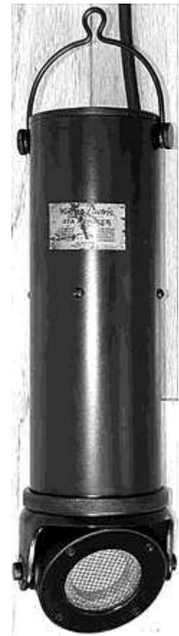
Right: Western Electric 47-A condenser microphone with a 394 "transmitter" (pre-amp) and "bail" clip for hanging attached on top, circa 1927. Widely used until the mid-1930s for cinema, radio broadcast, and studio recordings.
